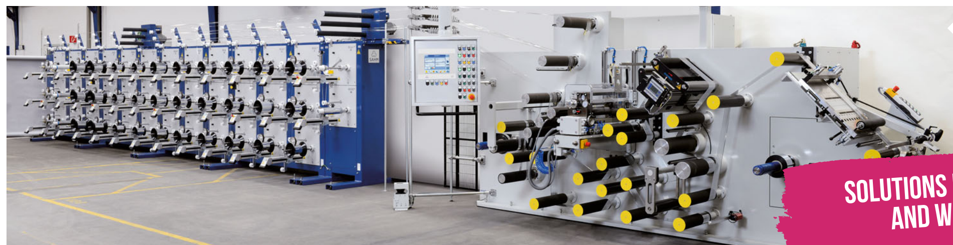
SAHM 411XE winders with an SSM 400 slitting machine from Adolf Müller GmbH und Co. KG.
